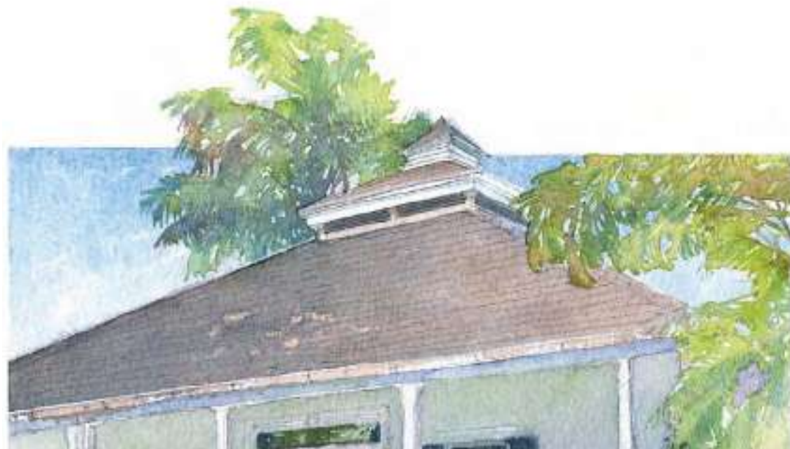
FIGURE 3.8- Roof incorporates cupolas to increase ventilation
