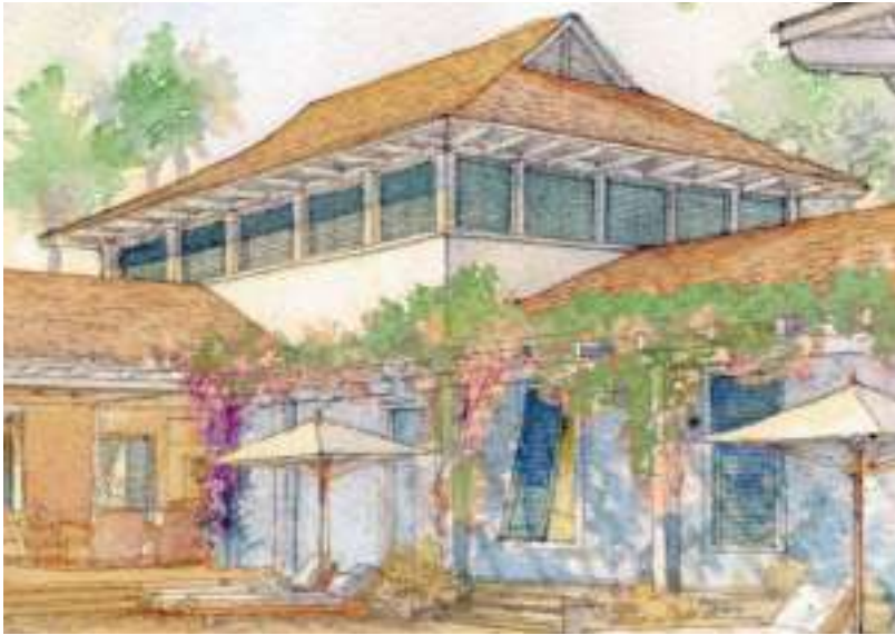
FIGURE 3.15 - Clareston windows allow for ventilation and increased daylighting opportunities.
